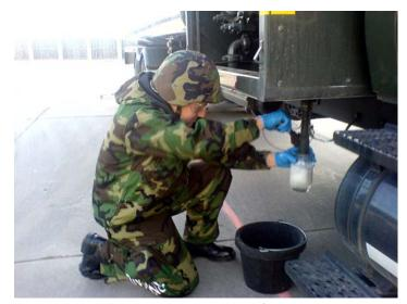
Staff Sgt. Joel Noell from the 507th Mission Support Groups Logistics Readiness Squadron's Petroleum, Oil and Lubricant (POL) section draws a sample from a fuel truck to conduct a visual examination.
